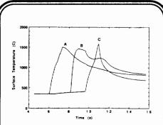
FIG. 5 Time histories of outboard divertor target surface temperature for ignited P<sub>fus</sub>=500 MW discharge and swept divertor. Maximum accumulated peaking factorsare assumed. Traces correspond to points at thebeginning (A), middle (B), and end (C) of the sweep trajectory.
