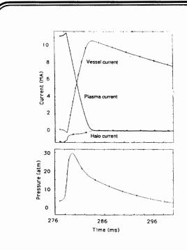
FIG. 3 a) Time histories of current during the disruption phase of a vertical displacement event. The disruption occurs ~ 60 cm below the midplane. The fast current decay (3 MA/ms) requires reduced halo temperatures during the disruption phase. b) Time history inboard vacuum vessel wall pressure.
