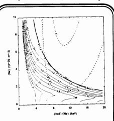
FIG. 1 CIT plasma operation contours (POPCON) for minimum-performance assumptions( $\tau_E$ =1.42xITER-P, 0.5% He). A conservative estimate of the beta limit,  $\beta$ =2I<sub>P</sub>/aB<sub>T</sub>, is used. With 20 MW of auxiliary heating, a fusion power of 100 MW and Q=5 is obtained, sufficient for burning-plasma physics studies. Solid contours: auxiliary power; dashed contours: Q.
